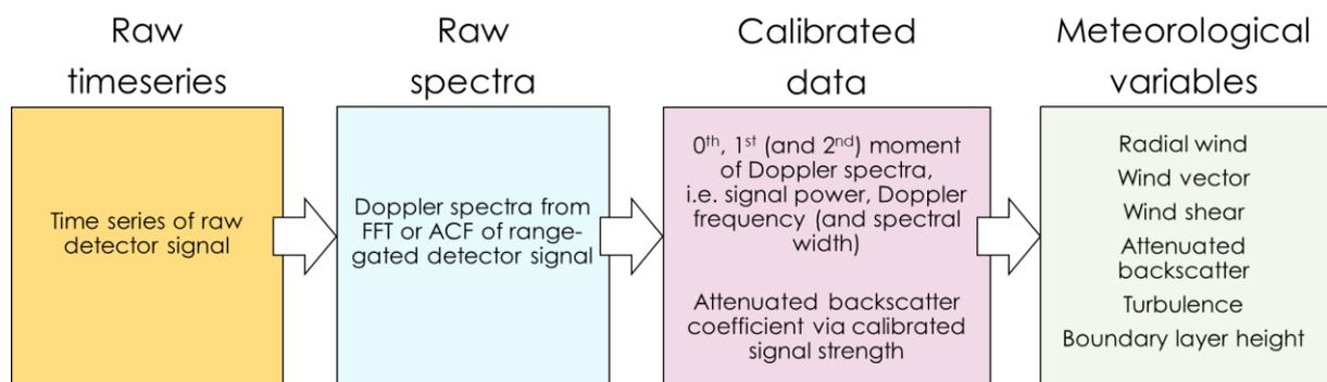
**Figure 1:** Processing steps for coherent (heterodyne) Doppler lidar systems
